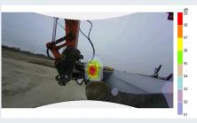
Noise sources that are moving, such as screen wipers, door slams and the moving arm of a crane, are more difficult to capture. The same goes for objects with changing operational conditions, such as starting up a powertrain, gear whine and brake squeal noise. Simcenter Sound Camera supports all such cases.
