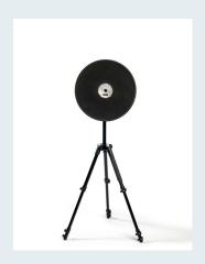
The Simcenter Sound Camera Digital Array is a modular, high-quality digital microphone array for sound source localization. It is an easy-to-set-up-and-use tool that helps both occasional users and engineers perform fast, accurate troubleshooting. The system has been designed to be a versatile solution, with arms that can be added or removed, making it an excellent tool to work with in multiple test conditions.
